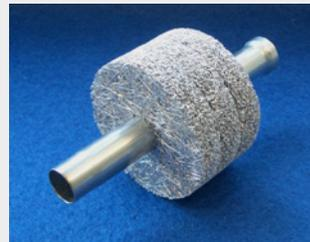
**Fig. 5:** Composite of tube and fiber structure. The distributed cavity in the structure is filled with the PCM. (Source: Fraunhofer IFAM)
