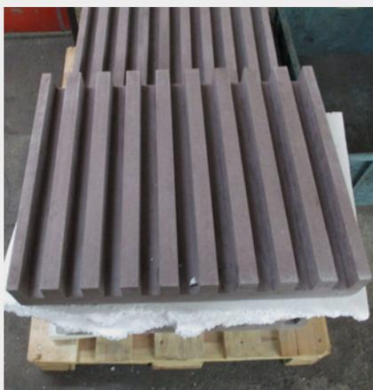
**Fig. 3:** Concrete storage tank for intermediate storage of residual heat. (Source: Hülsenbusch)
