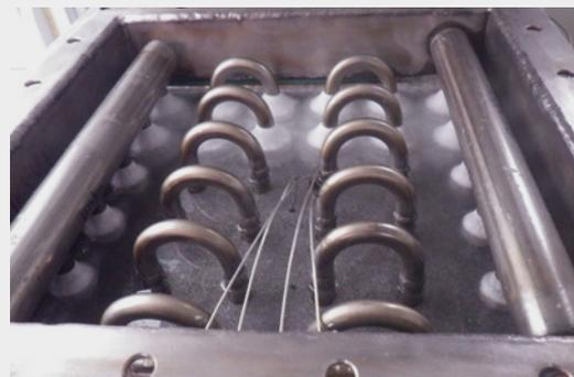
**Fig. 7:** Demonstrator for liquid heat transfer media. (Source: Fraunhofer IFAM)
